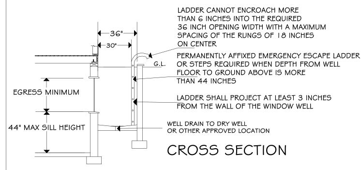
WINDOW WELLS USED FOR EMERGENCY EGRESS FROM BASEMENTS OR FLOORS LOWER THAN GRADE SHALL MEET THE FOLLOWING SIZE REQUIREMENTS FROM IRC SECTION 3 I O.2 THE MINIMUM HORIZONTAL AREA OF THE WINDOW WELL SHALL BE 9 SQUARE FEET, WITH A MINIMUM HORIZONTAL PROJECTION OF 36 INCHES. THE AREA OF THE WINDOW WELL SHALL ALLOW THE EMERGENCY ESCAPE AND RESCUE OPENING TO BE FULLY OPENED.
