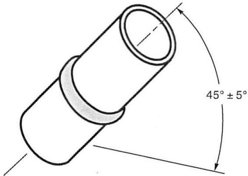
PIPE INCLINATION FIXED ( $45^\circ \pm 5^\circ$ ) AND NOT ROTATED DURING WELDING.
