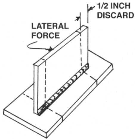
The fillet weld break specimen shall be cut from the test coupon as shown.
