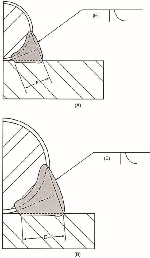
Note: Throat shall be measured as the shortest distance from the theoretical face to the point of fusion at the root as shown in dimension (E).
