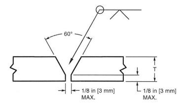
Note: T = qualification pipe or box tube wall thickness
