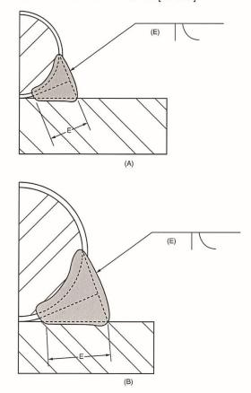
Note: Throat shall be measured as the shortest distance from the theoretical face to the point of fusion at the root as shown in dimension (E).
