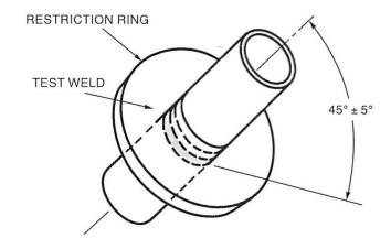
(E) MULTIPLE WELDING TEST POSITION 6GR WITH RESTRICTION RING (T-, Y-, OR K-CONNECTIONS)
