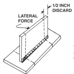
The fillet weld break specimen shall be cut from the test coupon as shown.
