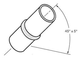
PIPE INCLINATION FIXED (45°  $\pm$  5°) AND NOT ROTATED DURING WELDING.
