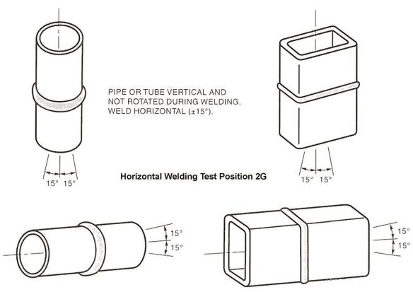
PIPE OR TUBE HORIZONTAL FIXED ( $\pm 15^{\circ}$ ) AND NOT ROTATED DURING WELDING WELD FLAT, VERTICAL, OVERHEAD.
